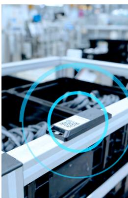
X-Tags - one of the smallest industry-specific UWB sensors. Its size and versatility allow for tracking even large quantities of objects.
